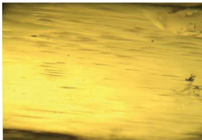
Figure 12b Etch pattern 20 Seconds for Cs - doped LAM crystals.
