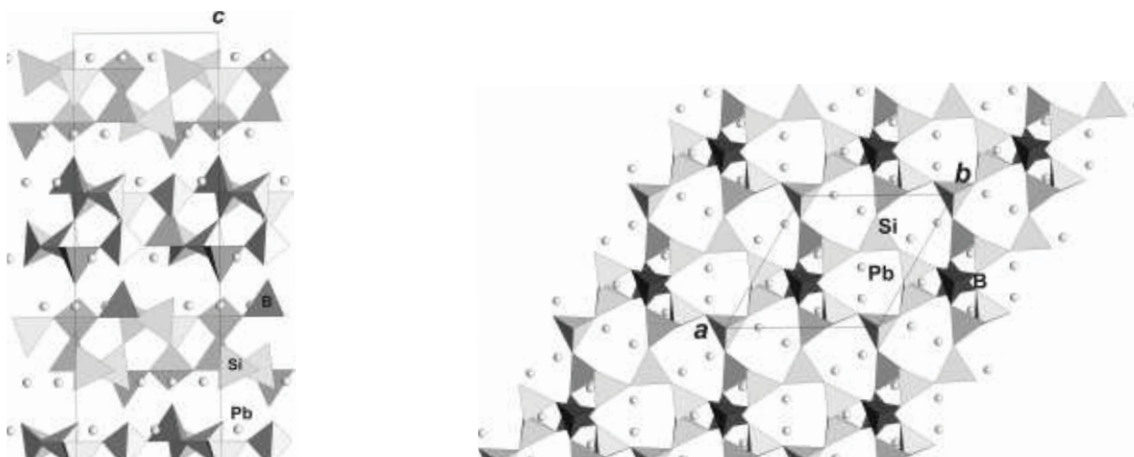
Figure 5 Projection of the structures \text{Pb}_{4.8}\text{Na}_{1.2}\text{Si}_8(\text{Si}_{1.2}\text{B}_{0.8})\text{O}_{25} onto ac plane (a), one double layer in ab -projection (b).
